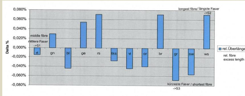
Cable with single-mode fibres – tensile test with fibre stretching
