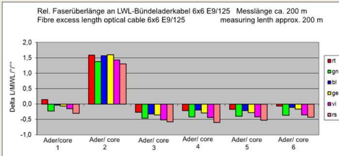
This should make it clear why there is basically no point in carrying out a tensile test with measurement of fibre stretching without measuring the excess length beforehand and identifying the longest, shortest and middle fibre.
