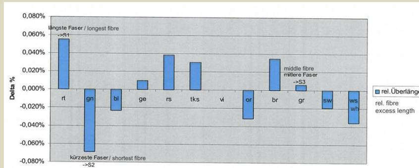
Cable with multimode fibres – tensile test with fibre stretching
