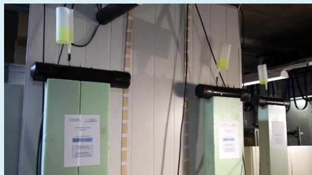
Test, 1.6 m water column
