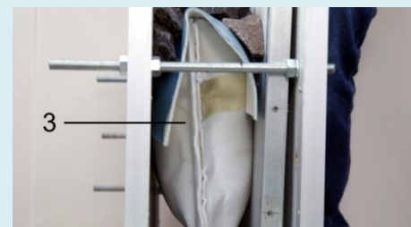
(3) 21.3 SVS-QADK/V S- Joint widths from 3 cm to \leq 16 cm
